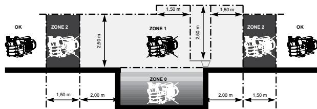
Install the pump in a dry, well-ventilated place. The motor requires the air to circulate freely around it to allow natural ventilation. Clear a space of at least 0.5m around the pump. Check regularly that no objects, leaves or other debris are blocking the motor cooling system.
